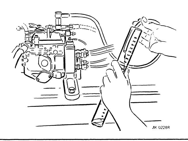
CHECKING DELIVERIES AND BREAKAWAY CHARACTERISTIC
